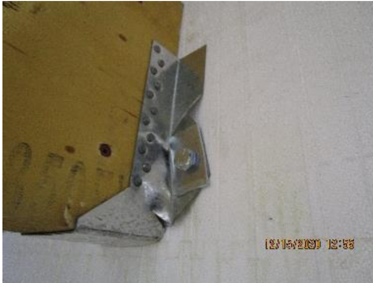
Photo No. 4 Typical ICF Joist Hanger Failure
