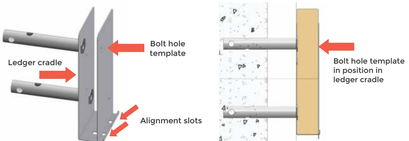
**IMPORTANT NOTE:** For drilling the holes in the wood ledger, use a **hole depth guide** so not to damage the threads of the cylinder bolt hole.
