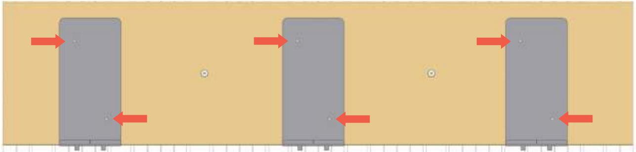
**5** Enlarge pilot holes using a 9/16" drill bit.
