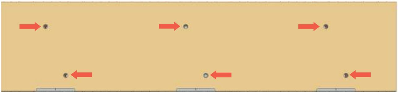
**6** Bolt the ledger board to the **BURMON-ICFWL** using the Hex Head bolts and washers supplied. Tighten securely.
